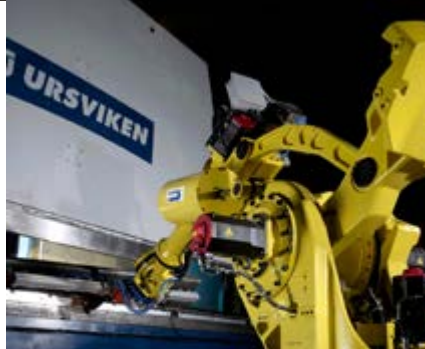
Robotic press handling system
