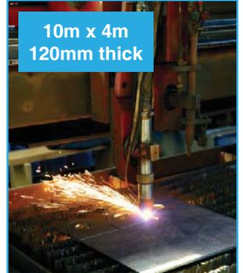
Flame cutting is ideal for cutting carbon steel and most metal alloys where cutting edge precision is not critical, or post machining is required.
