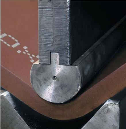
We specialise in cold forming and rolling steel and aluminium plates, a process involving zero heat input and does not affect the mechanical properties of the bent/ folded components.
