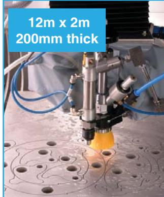
With four waterjet cutting machines available in-house, we can cut almost any materials up to 12m x 2m and 200mm thickness.
