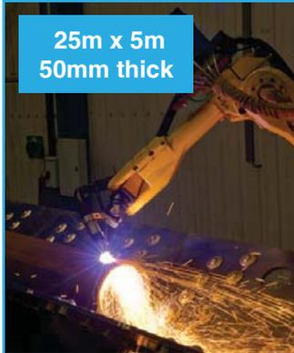
Our high definition plasma cutting technology with bevel capability has a large format cutting area of 25m x 5m with twin cutting head technology, allowing cutting of components up to 50mm thick.
