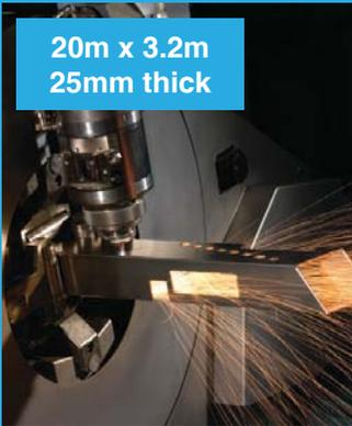
With 21 flat-bed lasers available in-house, we have the capability to cut parts up to 20m long x 3.2m wide in mild & stainless steel (25mm), aluminium (20mm), as well as copper & brass (10mm).
